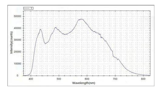
Figure 1 Output spectrum of ATG2000 ( Measure with ATP2000P spectrometer)
