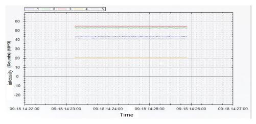
Figure 2 The output power stability of ATG2000 (change rate < 0.13%)
